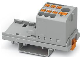
Distribution block, Block with vertical alignment and integrated supply, the blocks can be bridged with one another via the conductor shaft, for corresponding plug-in bridges, see accessories, nom. voltage: 690 V, nominal current: 24 A, connection method: Push-in connection, Push-in connection, number of connections: 7, cross section: 0.14 mm<sup>2</sup> - 4 mm<sup>2</sup>, AWG: 26 - 12, width: 28.6 mm, color: gray, mounting type: NS 35/7,5, NS 35/15
